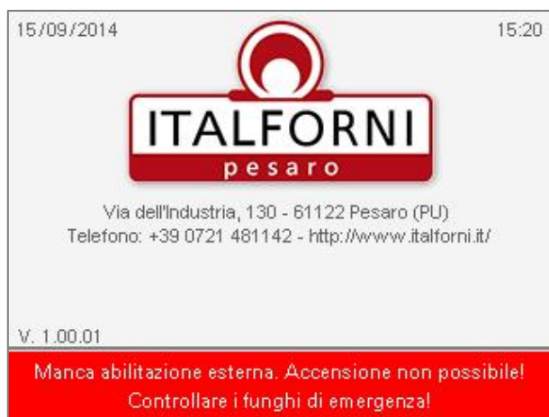
Fig.3 - Warning message for emergency mushrooms pressed
